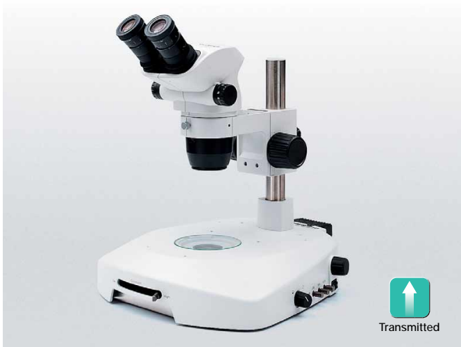
High-level transmitted light illumination base / SZX2-ILLB Provides effective contrast from oblique illumination and easily selected "High" and "low" contrast settings. Light volume and color temperature are adjusted by means of built-in filters (LBD/ND).
