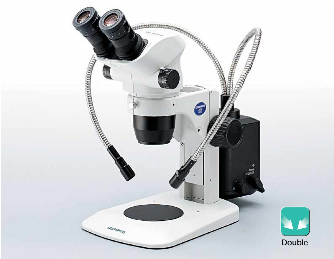
Interlock dual light guide / SZ2-LGDI Standard oblique semi-rigid fiber optic light guide. The light source position on the rear side of the stand saves desk space.
