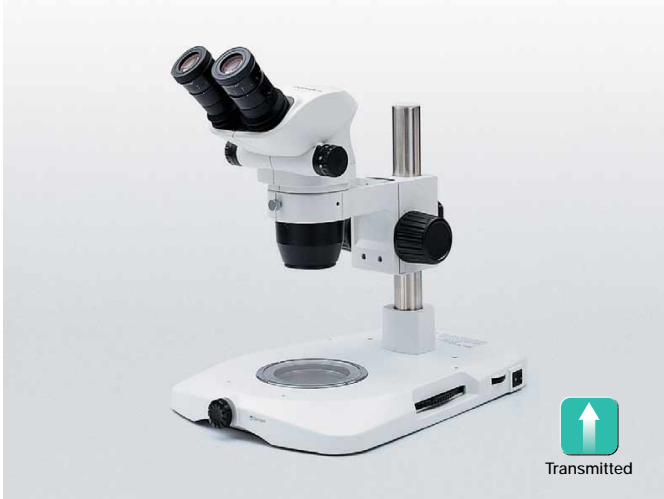
Slim LED transmitted light illumination base / SZX2-ILLT With a slim design of 41 mm, this transmitted light illumination base has a lower height to enable a low eyepoint and easy access to base-mounted samples during observation and operation. The LED 4-position turret enables contrast adjustment between brightfield, oblique, and darkfield illumination with a simple turn.
